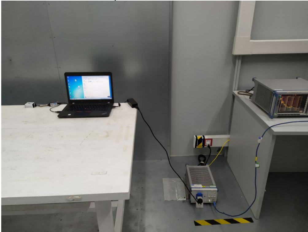
Photos of radiated emission test 30MHz – 1GHz
