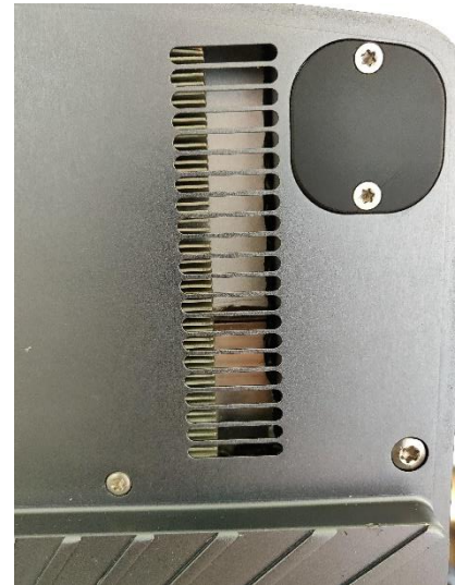
Figure 26 Air exhaust at the backside of antenna.
