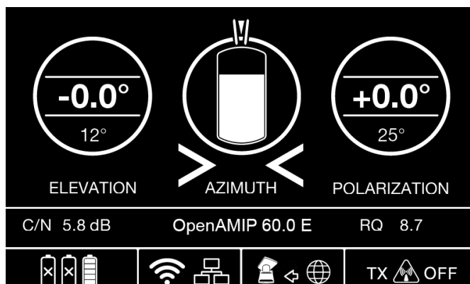
Figure 20 POINTING screen with current difference or offset from the absolute pointing value (0.0 for Elevation and Polarization both) in the middle of the two circles. The current value is the smaller number in the circles. Azimuth is aligned within the two bars on top of middle circle.
