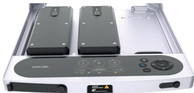
Figure 7 Connection ports are located on the front of the terminal. The DC power cable socket is located to the right. Ethernet and USB ports are located to the left.
