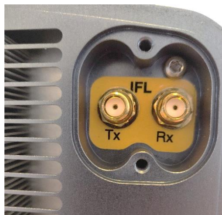
Figure C3b L-band interface, 50 ohms SMA connectors exposed.
