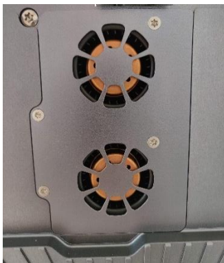
Figure 24 Fans behind fan cover.
