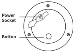
**Button** — ON/OFF. Push and hold 3 seconds to enter network configuration mode
