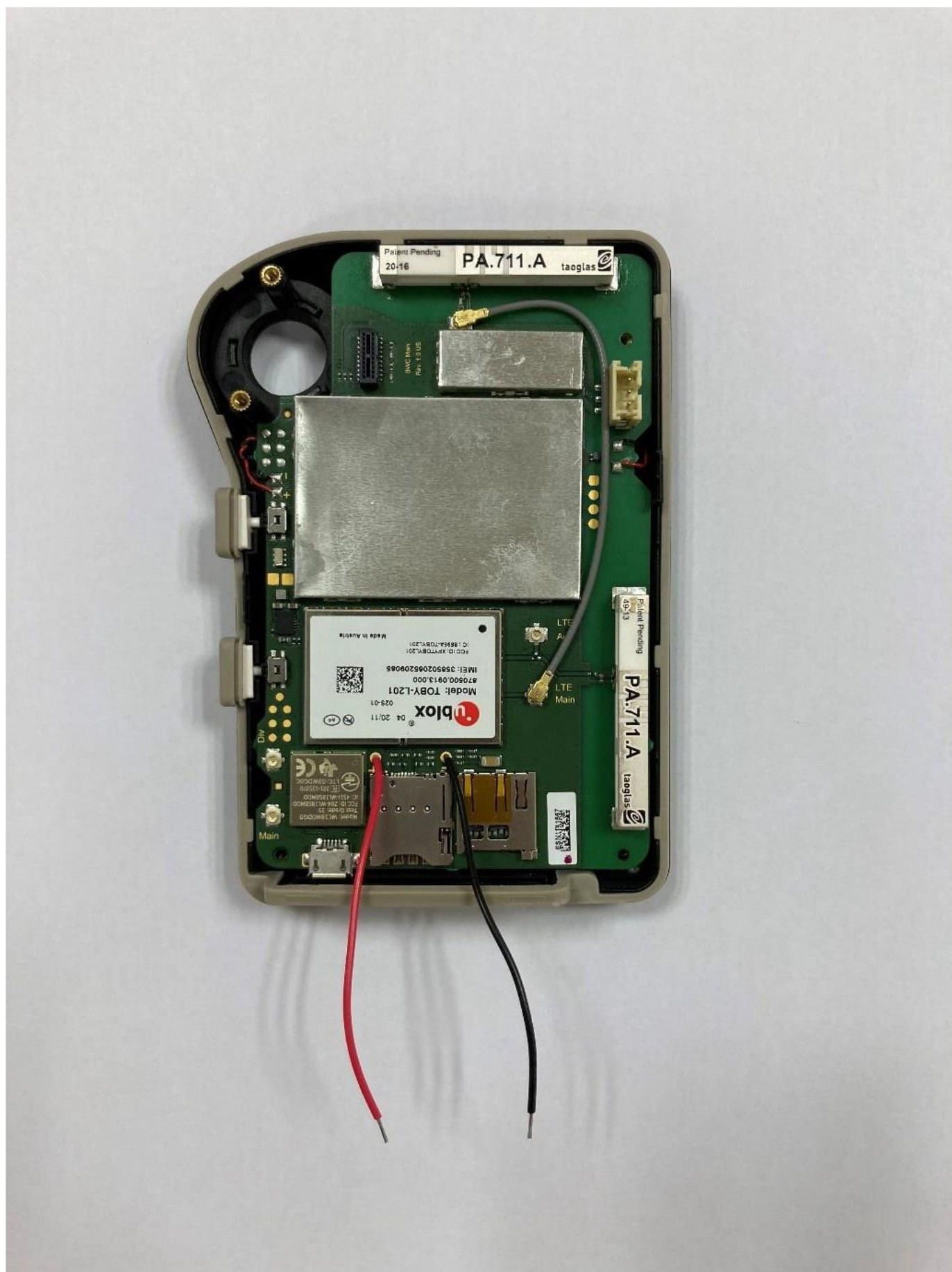
Front side Main PCB with EMC shield cans Fitted, installed in housing
