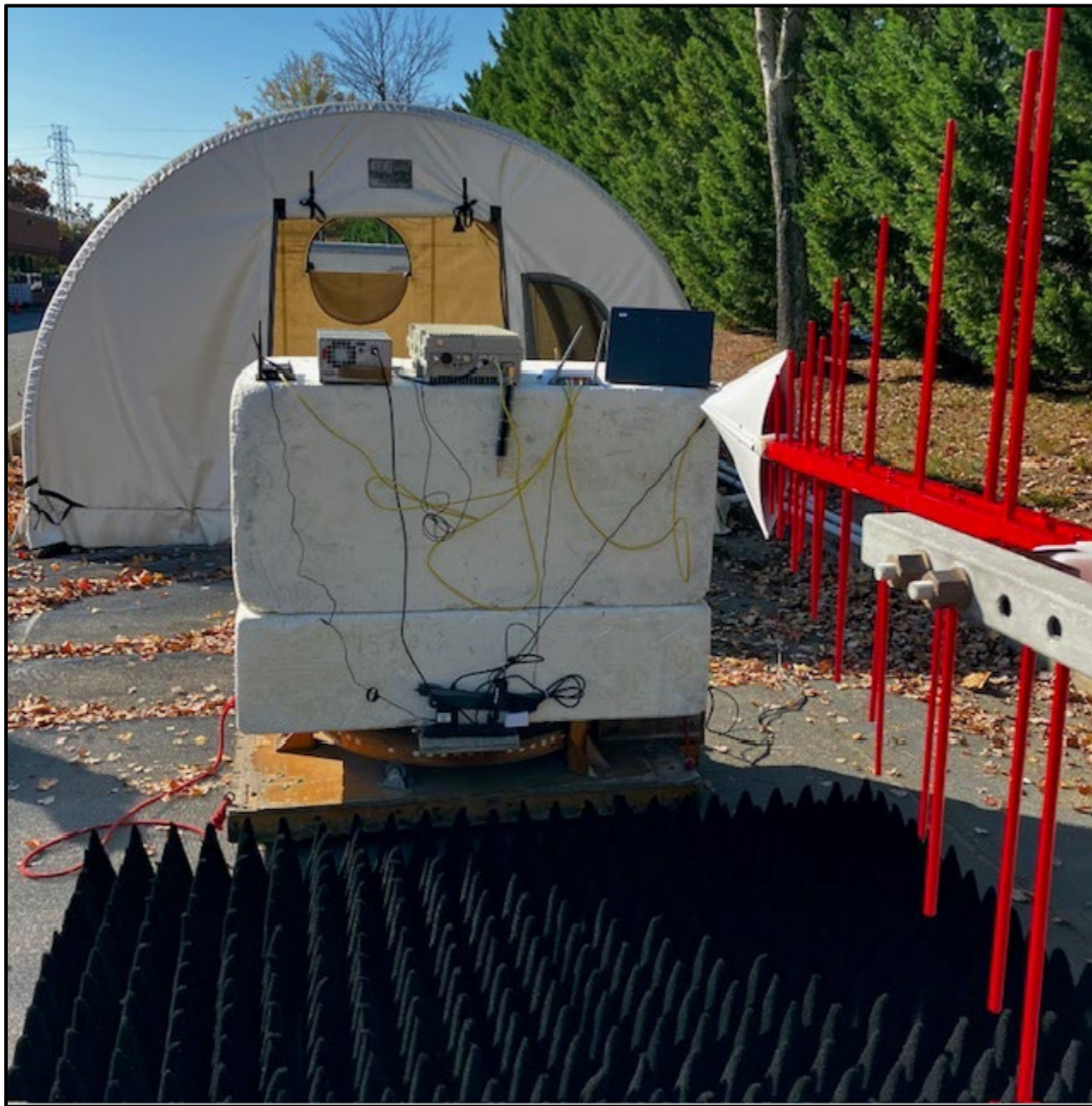
Photograph 4: Radiated Emissions – Back View (Above 1 GHz)
