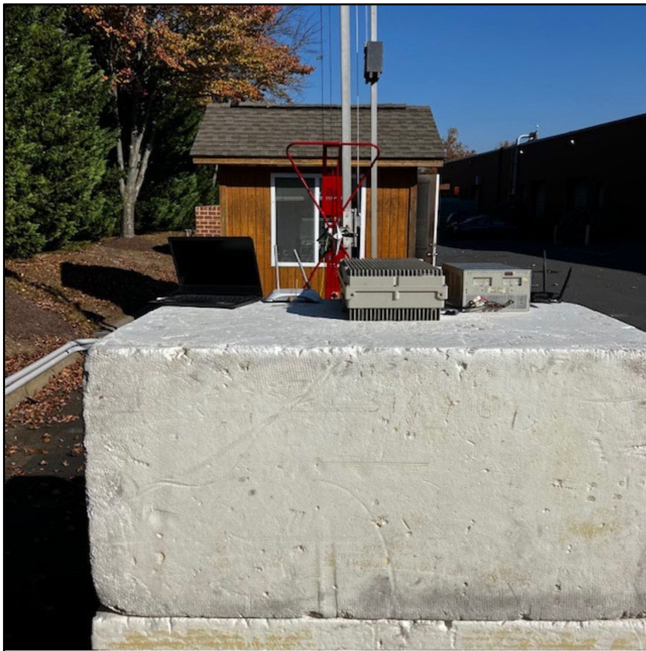
Photograph 3: Radiated Emissions – Front View (Above 1 GHz)
