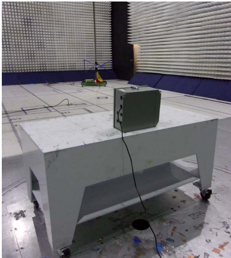
Electromagnetic Radiated Disturbance Setup Photograph
