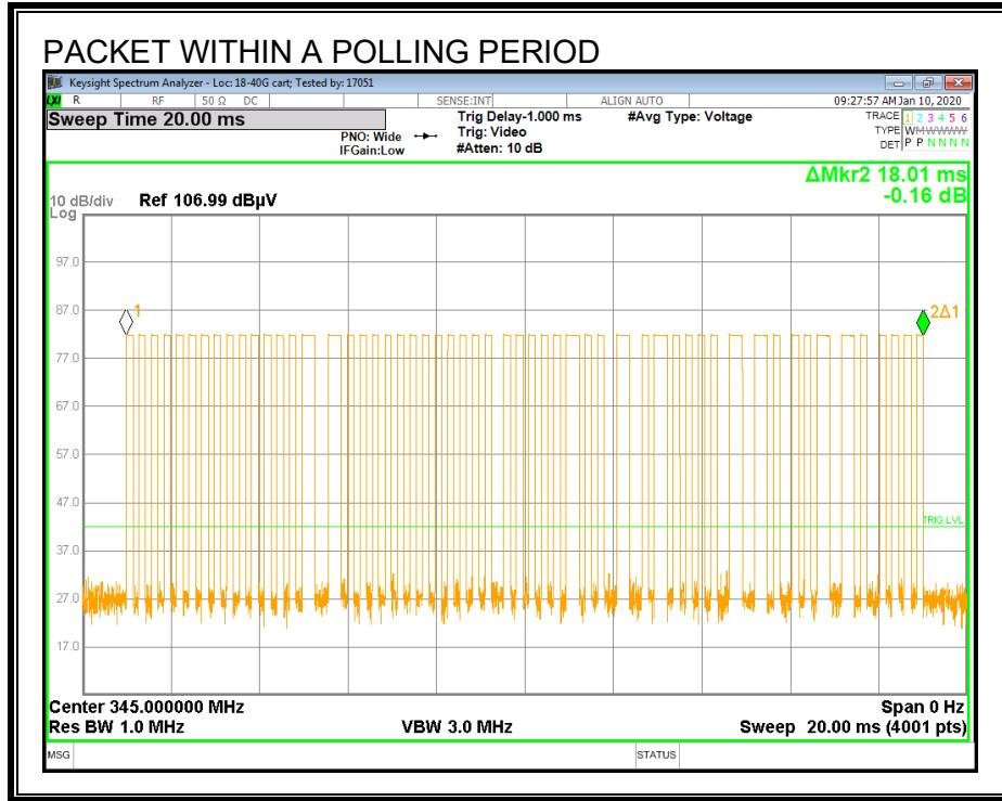
Worst-case packet size is 18.01ms. Therefore, EUT transmits 18.01ms within 60 min.
