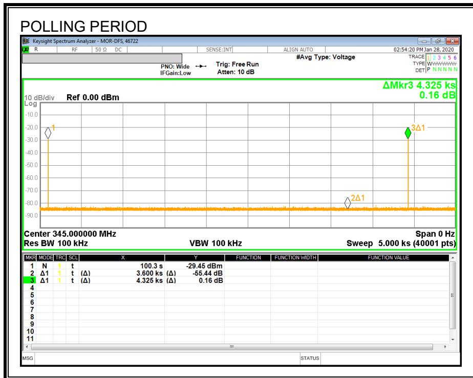
Marker 2 is at 60min. One packet transmitted within 60min.
