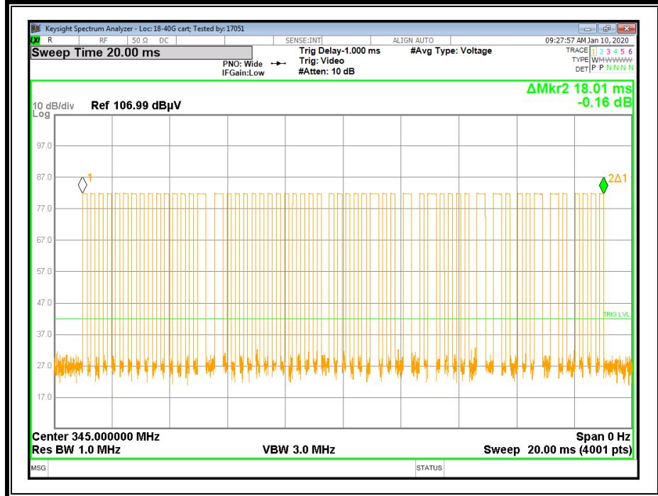
Note: Entire pulse width used as worst-case scenario vs. each short/long pulse width.
