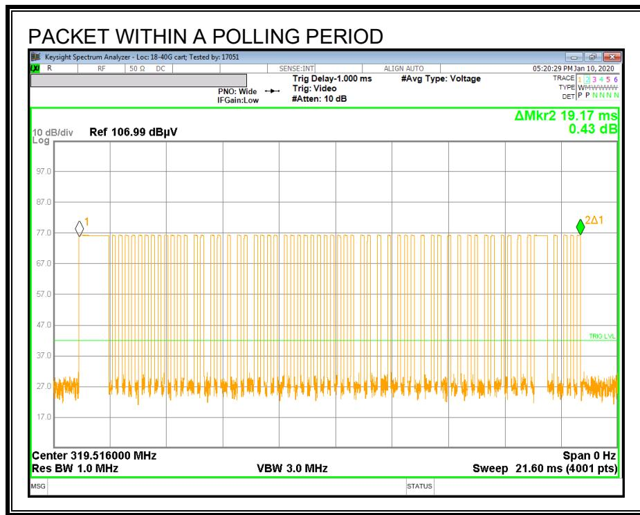
Note: Worst-case packet size is 19.17ms. Therefore EUT transmits 19.17ms within 60min.
