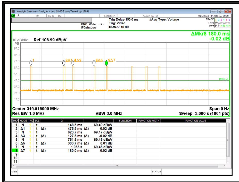
**NUMBER OF PULSES – MAGNET MOVING AWAY FROM EUT**
