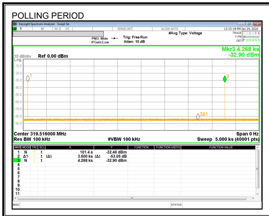
Note: Marker 2 at 60min. One packet transmitted within 60min.
