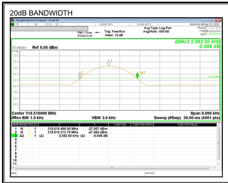
Note: Because the measured signal is CW or CW-like adjusting the RBW per C63.10 would not be practical since the measured bandwidth will always follow the RBW and the result will be approximately twice the RBW. See 99% OBW plot for 20 dB BW measurement relative to the RBW.
