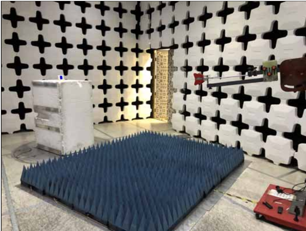
Test Setup for Radiated Spurious Emissions: Above 1GHz, Horizontal Polarization
