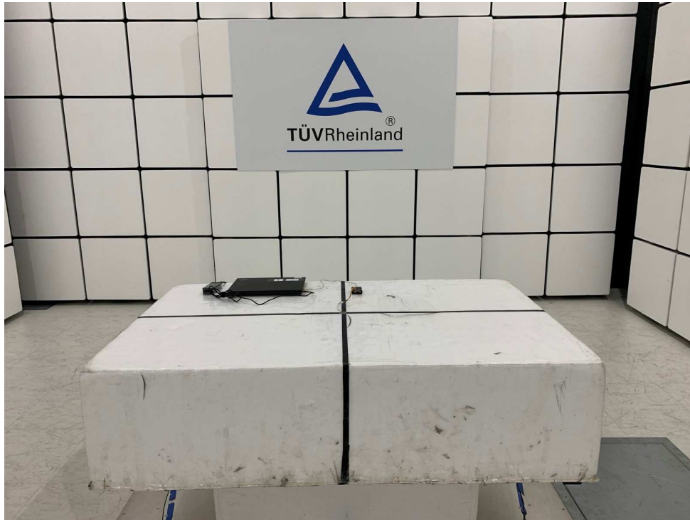
Photograph 1: Set-up for Spurious Emissions (Front View 1)
