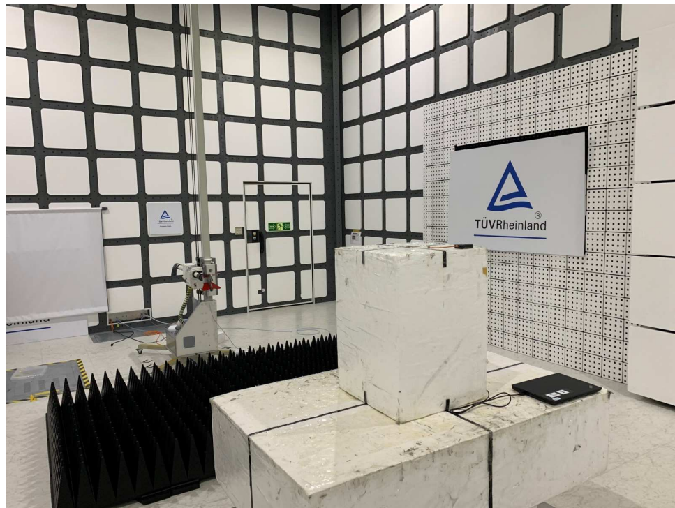
Photograph 4: Set-up for Spurious Emissions (Back View 2)
