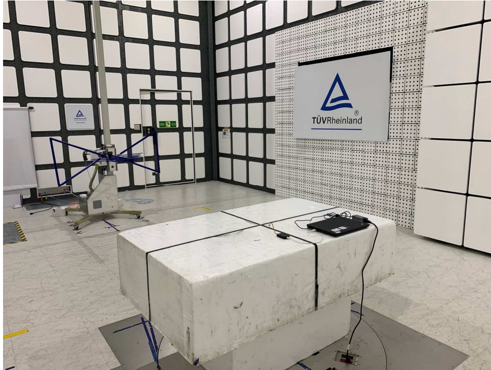
Photograph 3: Set-up for Spurious Emissions (Back View 1)
