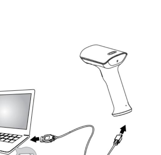
1) Connect the device interface (type-C interface) of USB to scanner;
