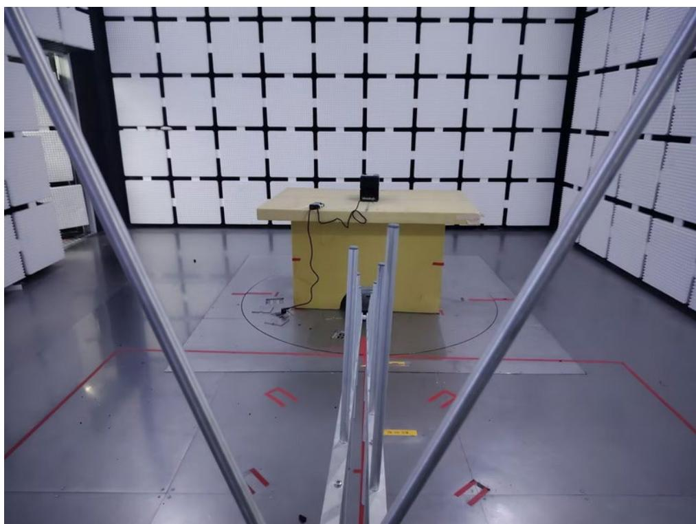
**Radiated Emissions Test Photos****1 GHz to 18GHz**
