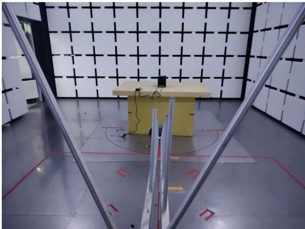
**Radiated Emissions Test Photos****1 GHz to 18GHz**
