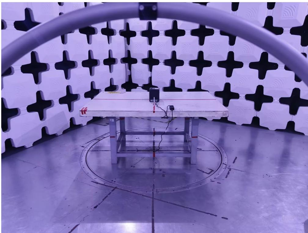
**Radiated Emissions Test Photos****30 MHz to 1000 MHz**
