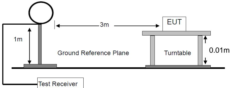
For Radiated Emission 30-1000MHz
