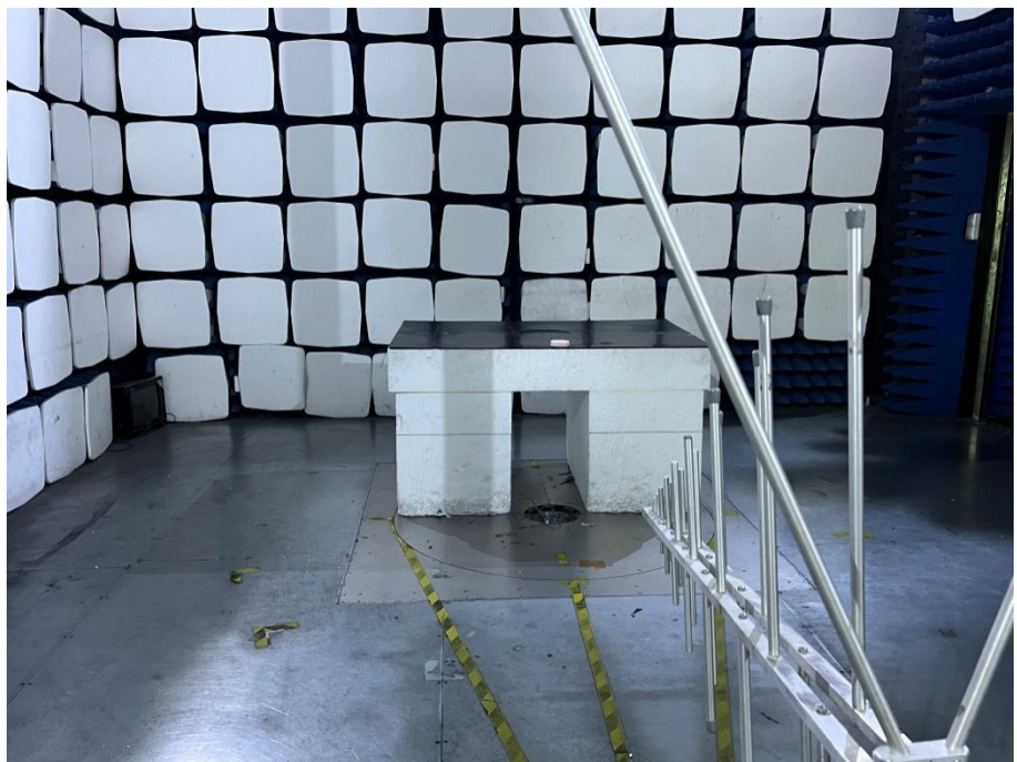
Radiation Emission Test Setup (30MHz to 1GHz)
