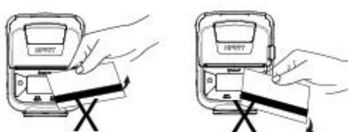
If you extract a card at the end of the MSR slot by lifting up or lowering down, the card is not maintained and a read error occurs.
