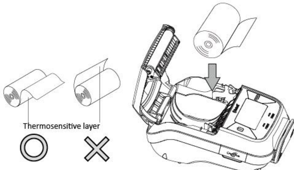
3) Pull the end of the roll straight toward you. Then press down on both sides of the printer cover to close it firmly. When you close the printer cover, make sure that it is closed on both sides.
