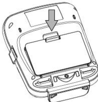
3. To remove the battery pack, pull back the hook, and use the opposite procedure from the one you used to insert the battery pack.
