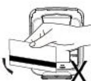
If you insert a card into the middle part of the MSR slot, the card is not read correctly and read error occurs, or if you move the card back or forth by force after inserting into the MSR slot, the card is not read correctly and a read error occurs.
