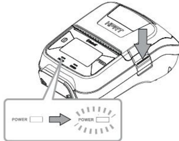
2. Press and hold both the MODE & FEED. Release the buttons after printer displays "Enter Menu Mode", then you can configure the settings.
