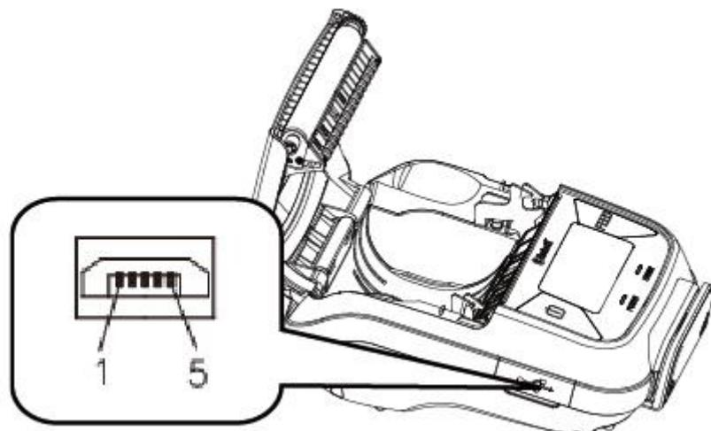
HM-E300 printer has a USB interface for Battery charging and is connected by means of 5pin micro USB socket. In the following table, the signals present on the micro USB socket are listed.
