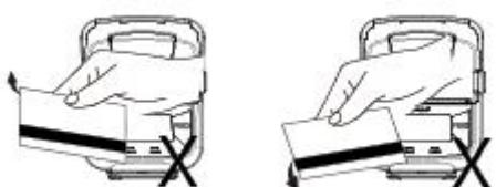
If you insert a card tilted upward/downward into the MSR slot, the card does not move horizontally and a read error occurs.
