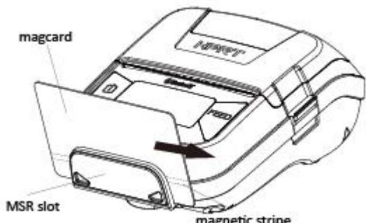
Make sure the magnetic stripe is towards to the magnetic head. Hold the card in the center as illustrated below and swipe it straight at a steady speed in the direction of arrows.
