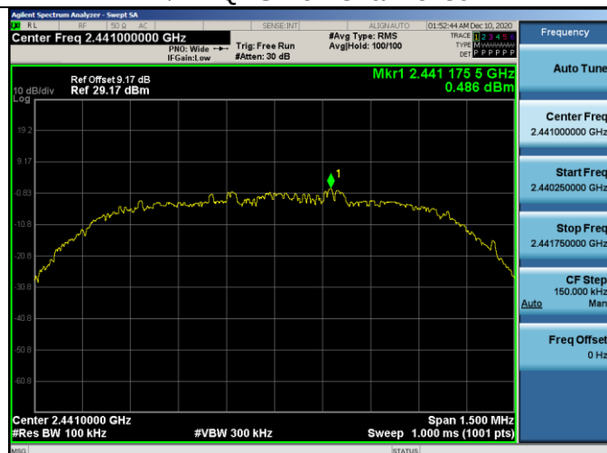
\pi/4 -DQPSK on Channel 39
