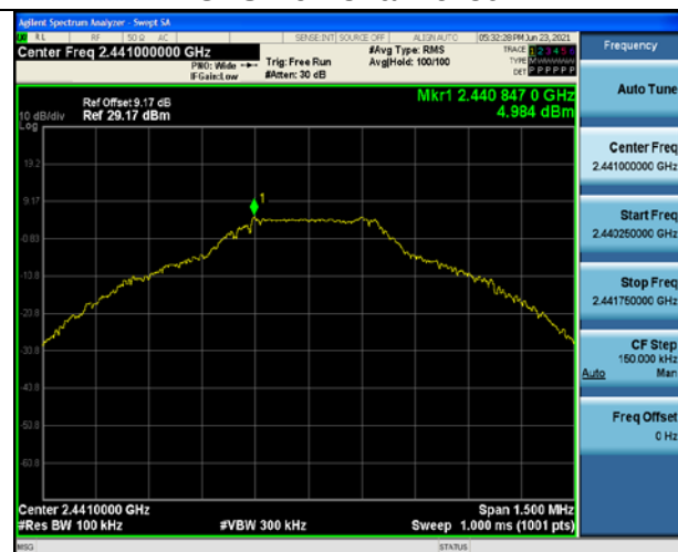
GFSK on Channel 39
