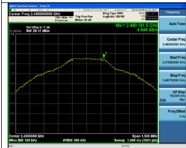
GFSK on Channel 78
