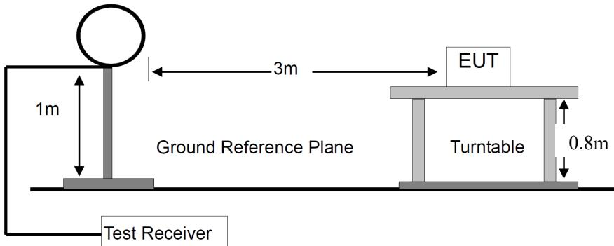
For Radiated Emission 30-1000MHz
