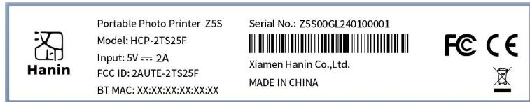
Specifications: The label shall be securely affixed to a permanently attached part of the device, in a location where it is visible or easily accessible to the user, and shall not be readily detachable. The label shall be sufficiently durable to remain fully legible and intact on the device in all normal conditions of use throughout the device's expected lifetime.
