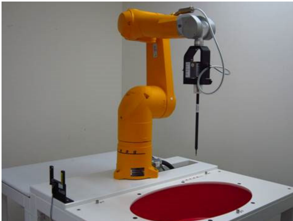
Fig.1 Photograph of the SAR measurement system
