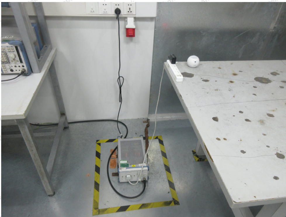
Photo of Conducted Emission Measurement
