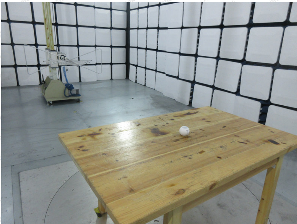
Photo of Radiation Emission Test
