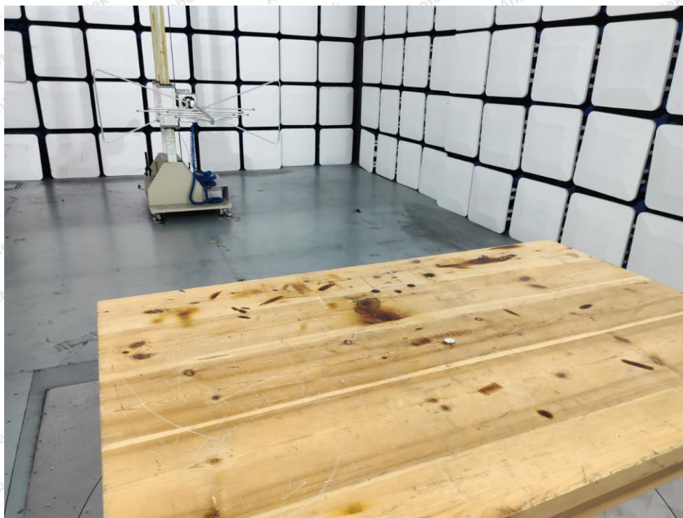
Photo of Radiation Emission Test
