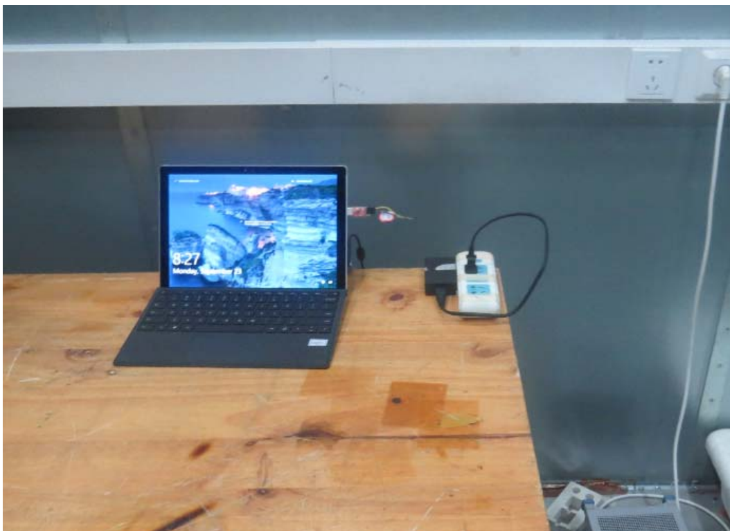
Picture 2 Conducted Emission Test Setup
