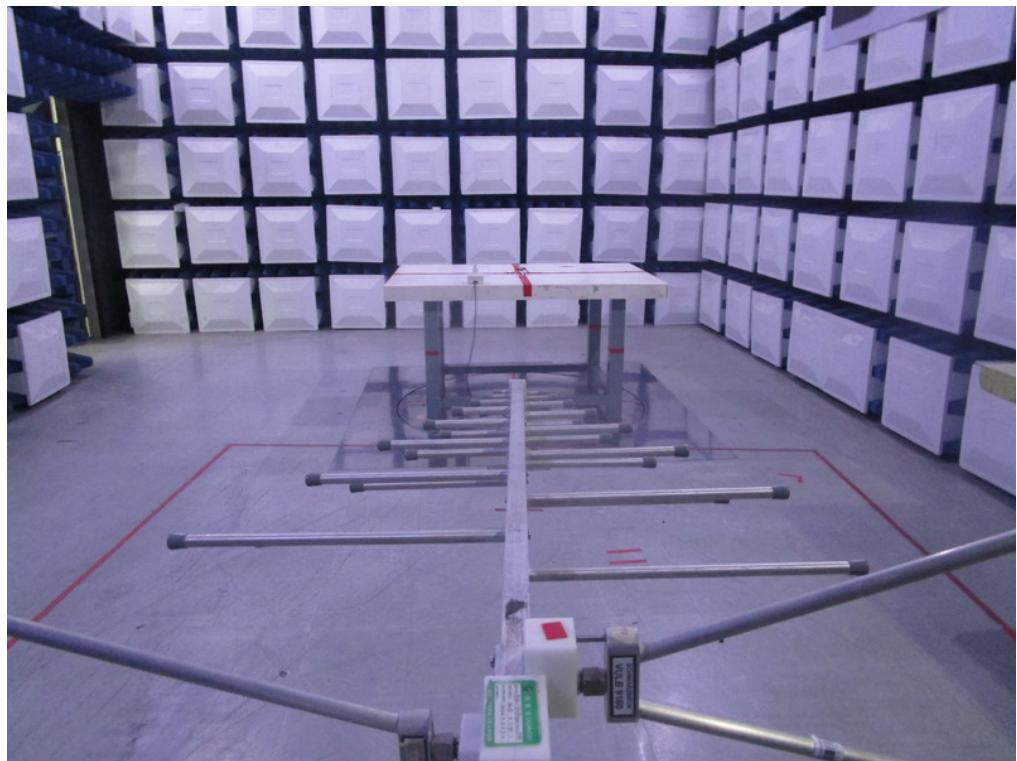
**Radiated Emissions Test Photos****Above 1 GHz**
