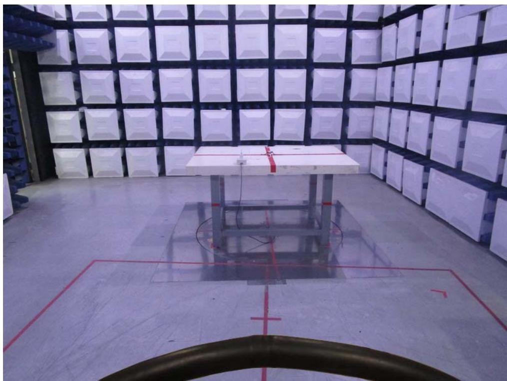
**Radiated Emissions Test Photos****30 MHz to 1 GHz**
