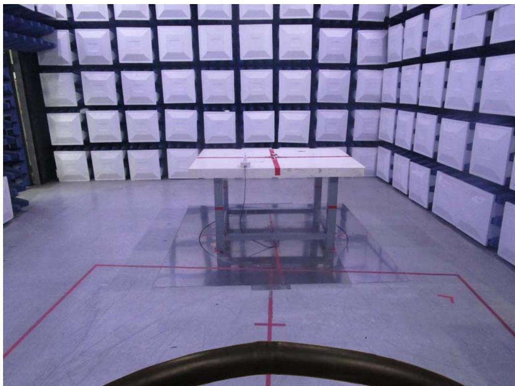
**Radiated Emissions Test Photos****30 MHz to 1 GHz**
