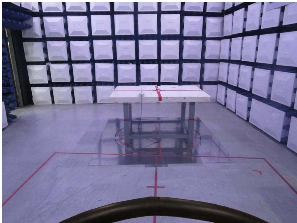
**Radiated Emissions Test Photos****30 MHz to 1000 MHz**
