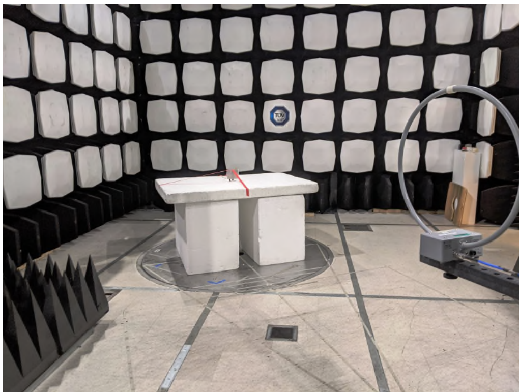
Figure 2: Equipment Under Test – Radiated Emissions <30MHz
