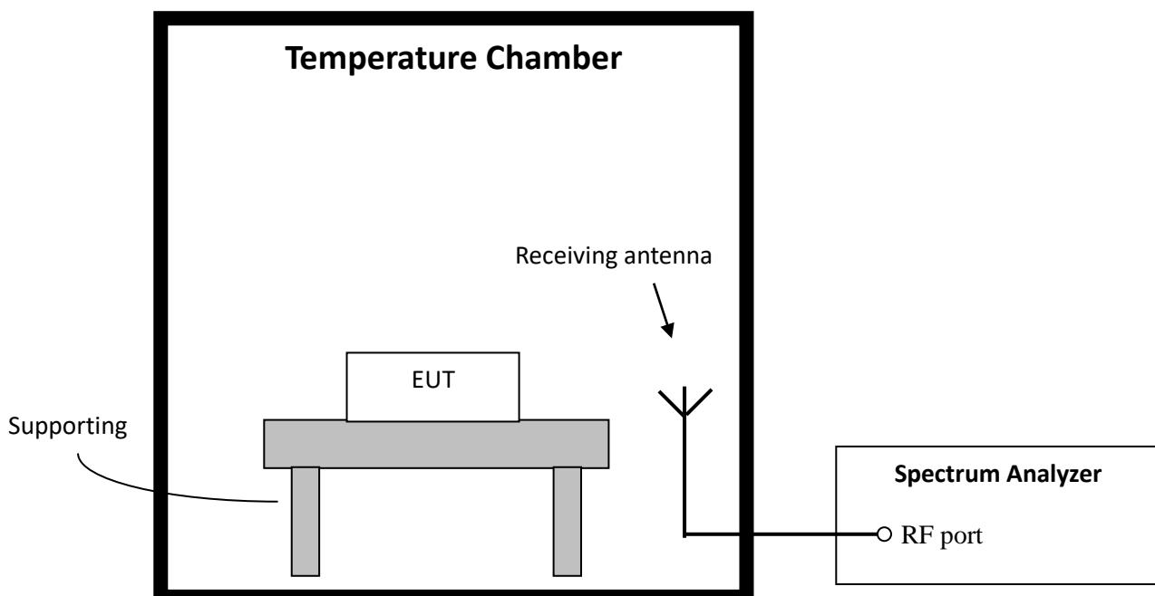
**TEST REPORT****5.3 Test procedure and test setup**
