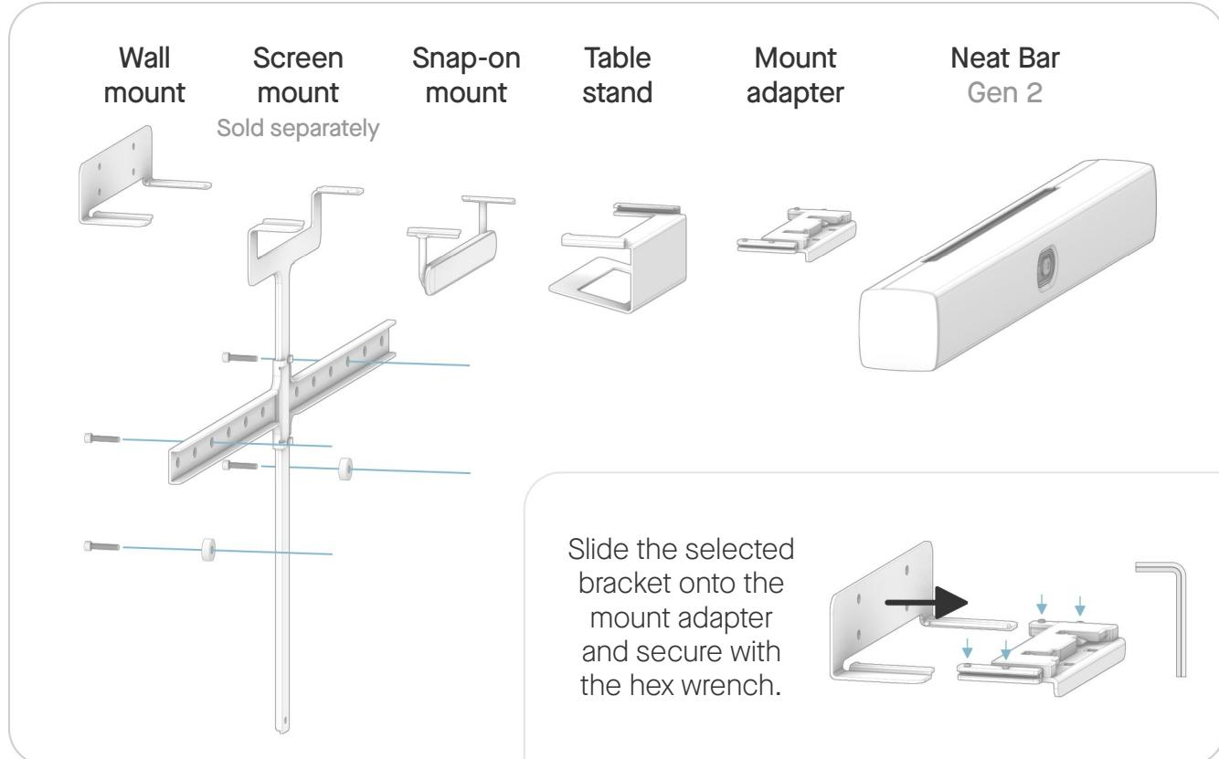
Slide the selected bracket onto the mount adapter and secure with the hex wrench.
