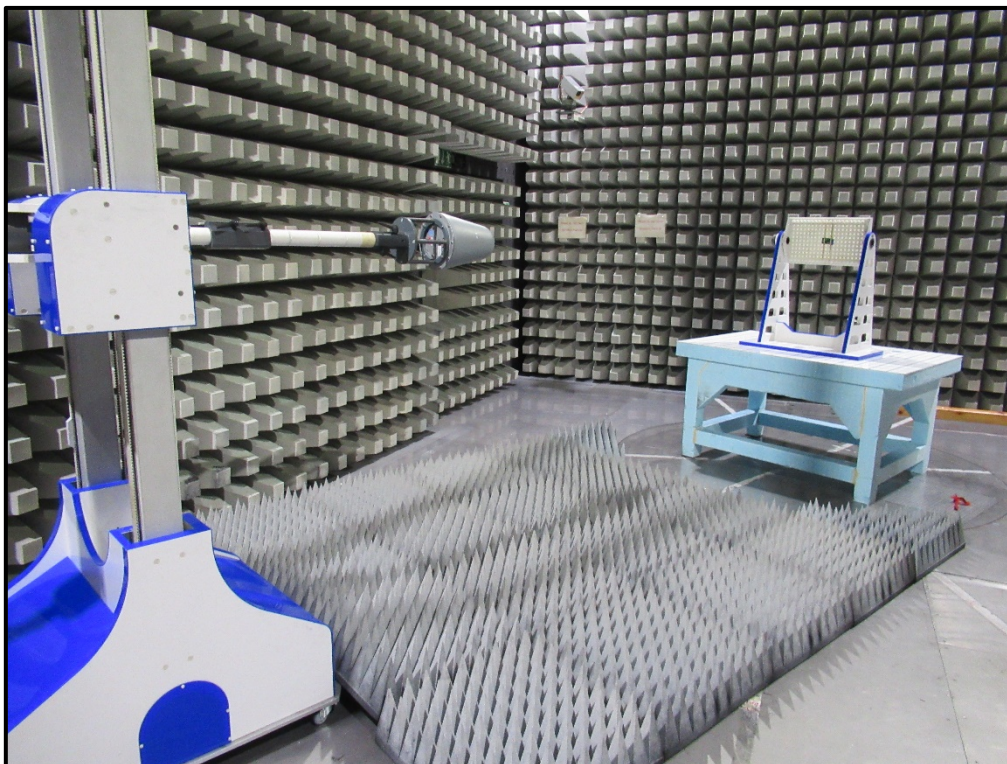
Photo 5: Radiated Test Setup -1 GHz to 10 GHz
