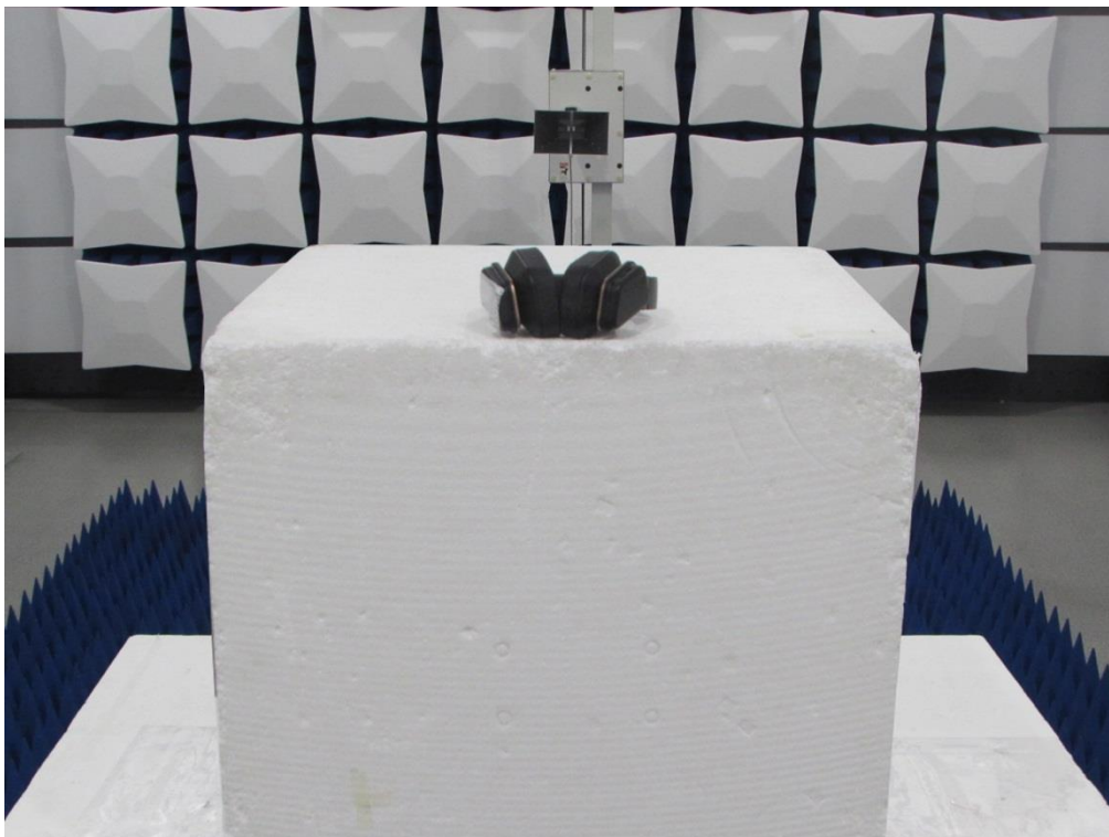
Radiated Emission Above 1GHz
