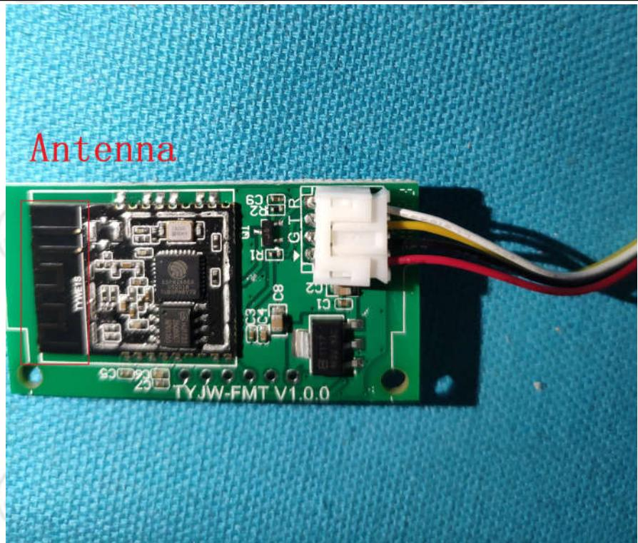
The antenna is integrated on the main PCB and no consideration of replacement. The best case gain of the antenna is 3dBi.
