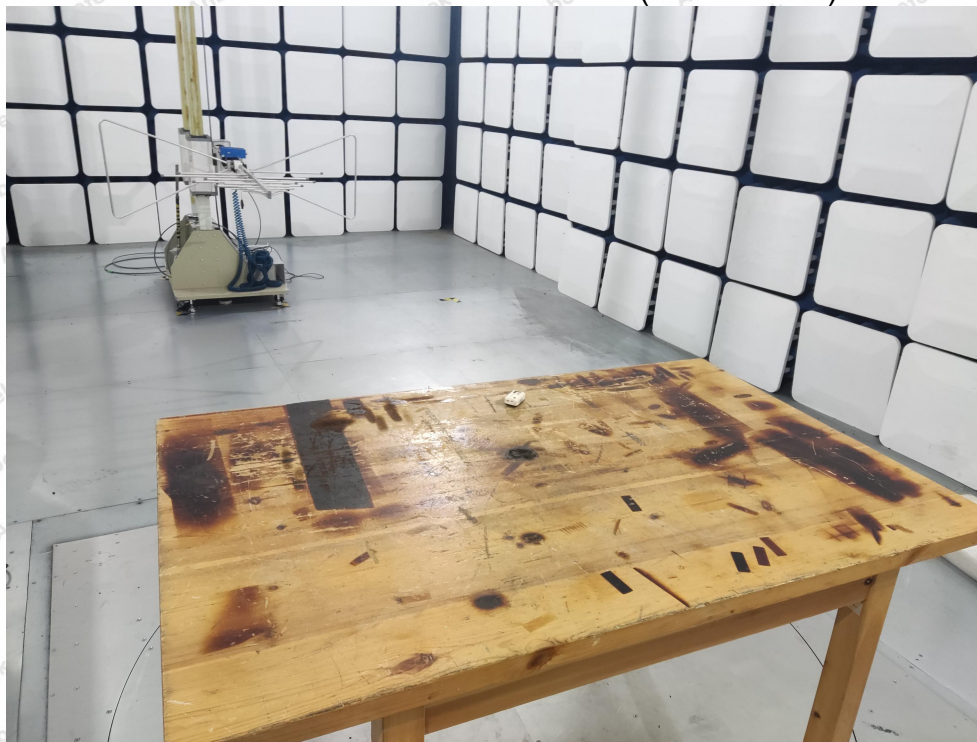
Photo of Radiation Emission Test (Below 1GHz)
