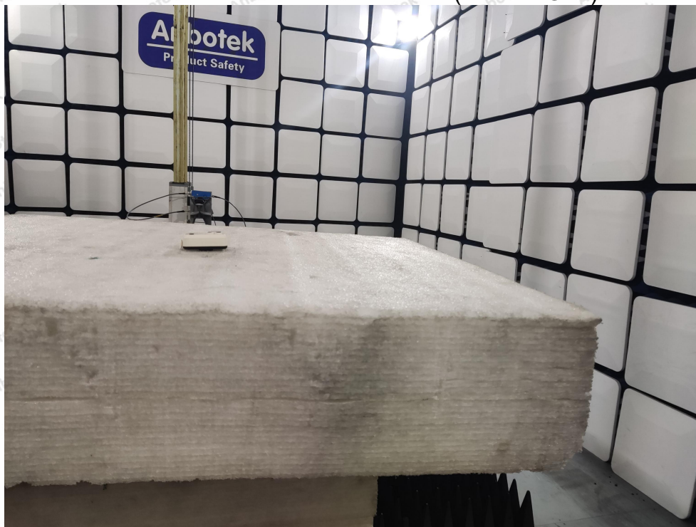
Photo of Radiation Emission Test (Above 1GHz)
