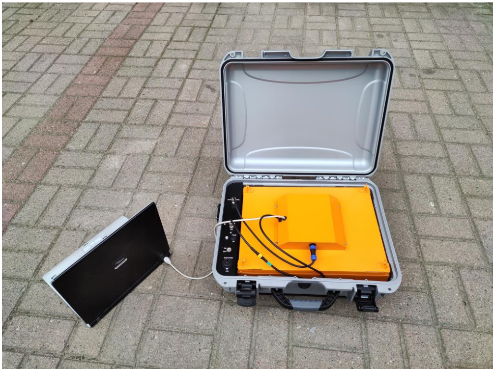
Fig.2. Zond Aero 500 GPR in the shockproof case.
