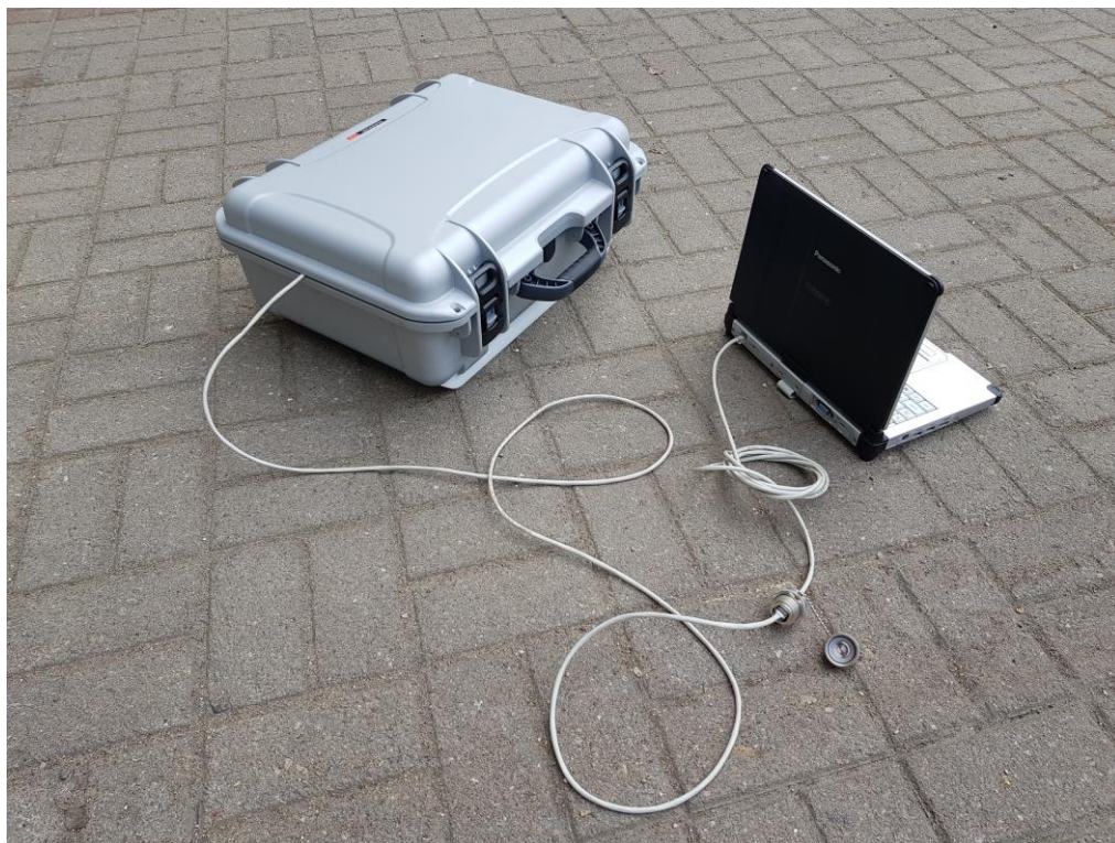
Fig. 8. Zond Aero 500 GPR data acquisition.
