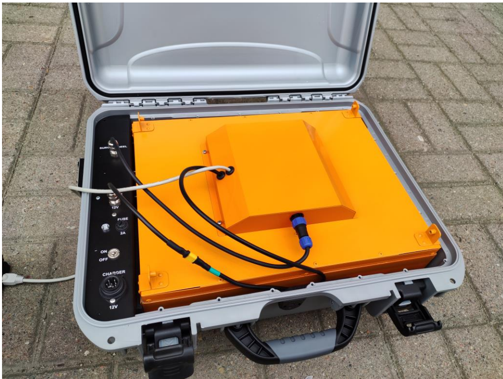
Fig.3. View of shock proof case control panel with mounted Zond Aero 500 GPR.
