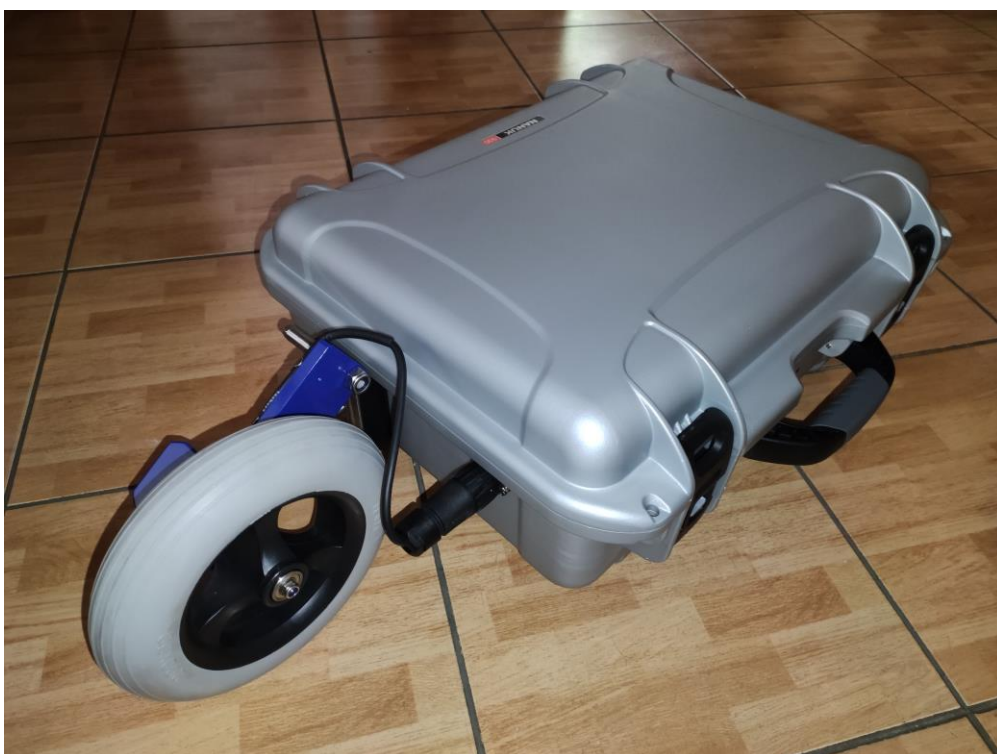
Fig.4. Survey wheel mounted on the shock proof case.
