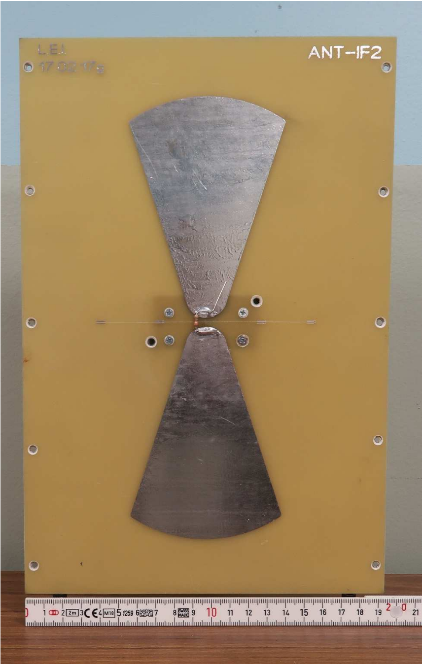
Rx Antenna Front
