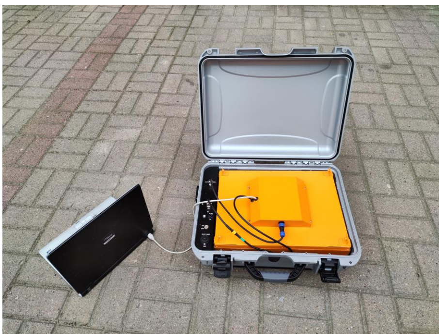
Fig.2. Zond Aero 500 NG GPR in the shockproof case.
