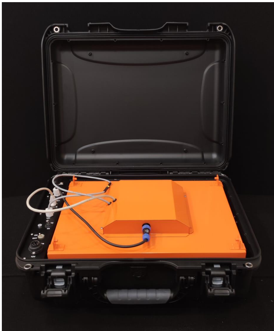
Fig.3. View of shock proof case control panel with mounted Zond Aero 500 NG GPR.
