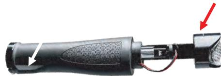
The turn signal lights are powered by a "AAA" battery in each grip. To change the batteries, loosen the set screws at either end of the grip.
