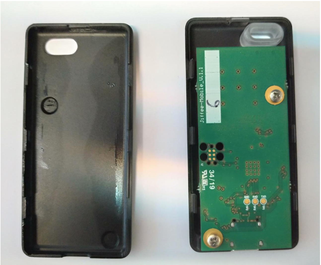
Picture 1. Jiffee Dongle - Mobile Version - without bottom cover
