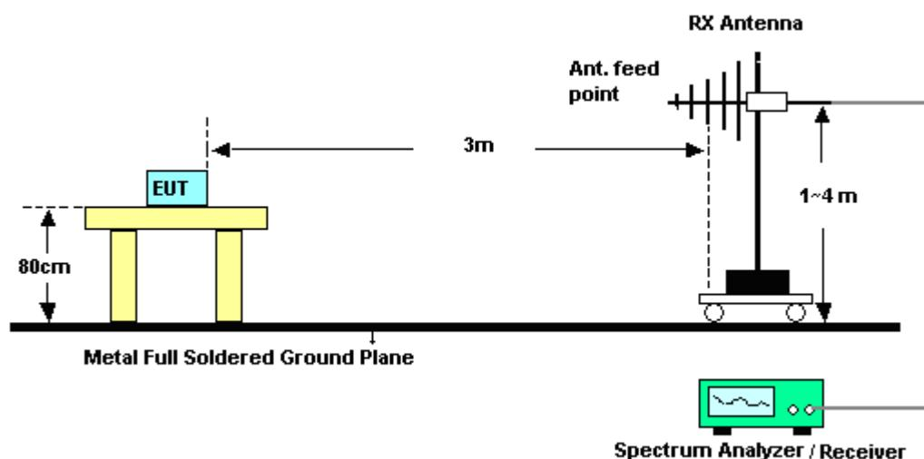
**For radiated emissions above 1GHz**
