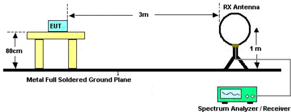
For radiated emissions from 30MHz to 1GHz
