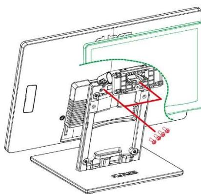
Step 2: insert the display arms and screw them on. (4 screws are provided with the optional display.)
