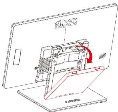
Step 2: unscrew and separate the stand from the display.
