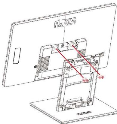
Step 3: secure VESA by screwing it on.
