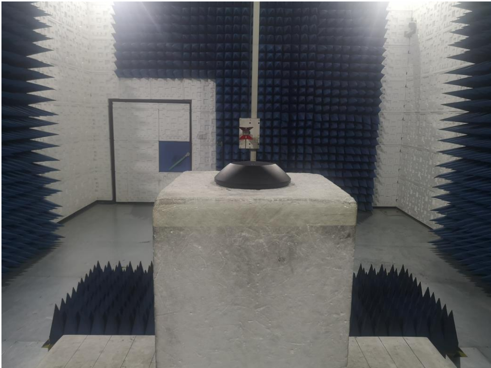
RADIATED EMISSION TEST SETUP ABOVE 1GHZ
