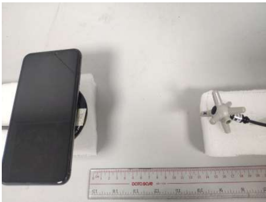
E-field Test Setup Photo Positon D(15cm)
