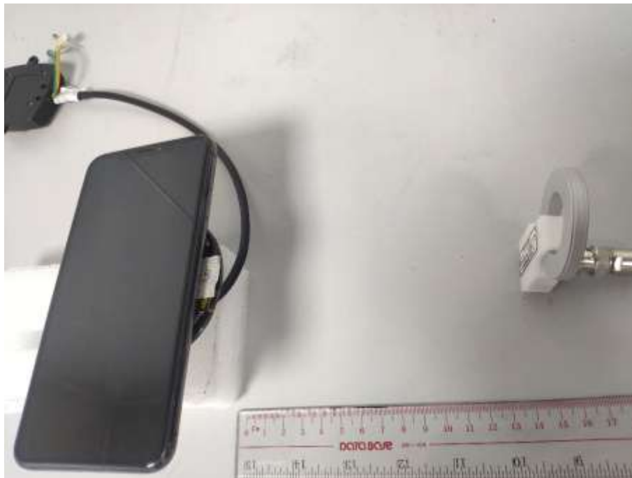
H-field Test Setup Photo Positon B(15cm)
