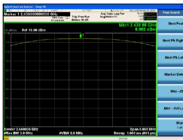
GFSK (BLE 2Mbps) MIDDLE CHANNEL
