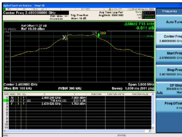
GFSK (BLE 1Mbps) HIGH CHANNEL
