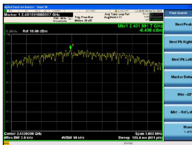
GFSK (BLE 1Mbps) LOW CHANNEL
