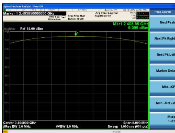
GFSK (BLE 2Mbps) LOW CHANNEL
