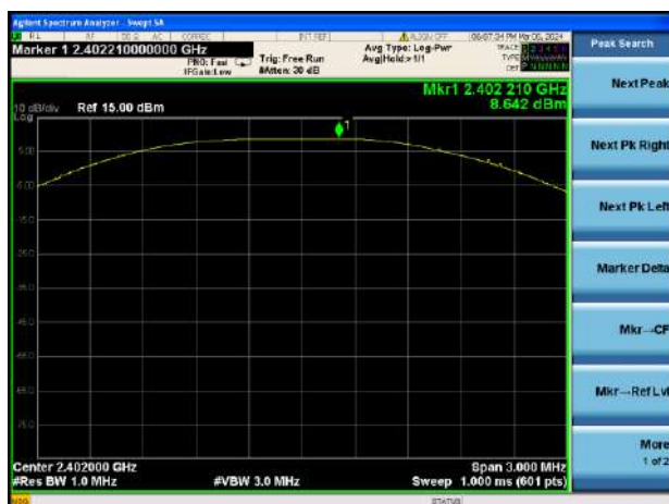
GFSK (BLE 1Mbps) LOW CHANNEL
