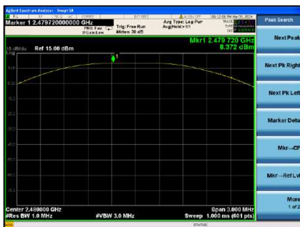
GFSK (BLE 1Mbps) HIGH CHANNEL
