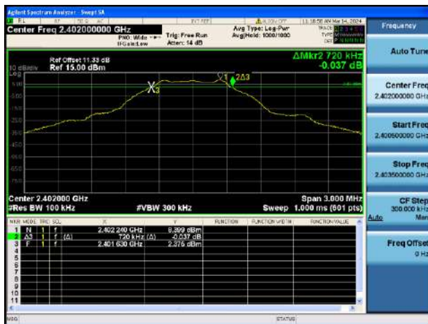
GFSK (BLE 1Mbps) LOW CHANNEL
