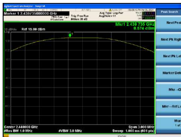
GFSK (BLE 1Mbps) MIDDLE CHANNEL
