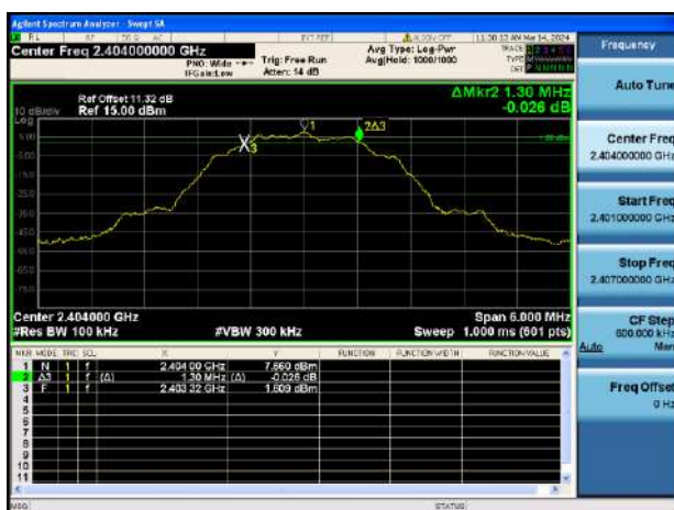
GFSK (BLE 2Mbps) LOW CHANNEL
