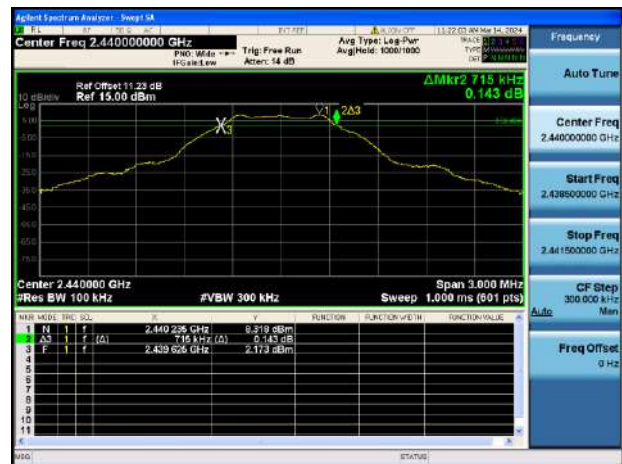
GFSK (BLE 1Mbps) MIDDLE CHANNEL
