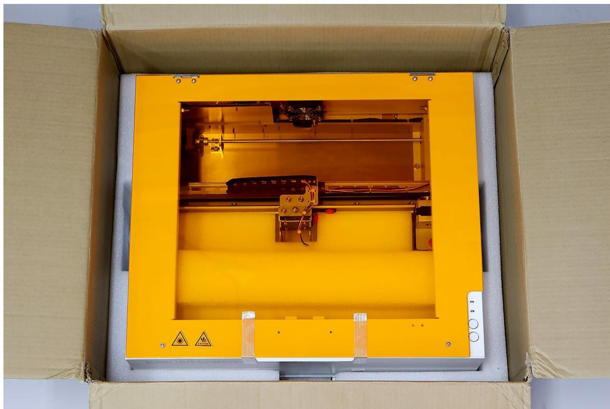
Carefully remove the device from the box and place it on a flat and level surface. Please make sure that nothing is blocking the exhaust fan on the back side of the device and keep the main unit at least 7inch away from anything behind the device (walls, etc.).
