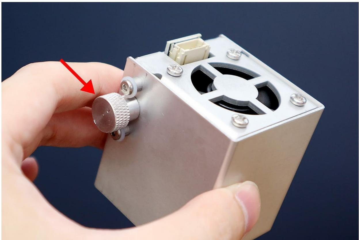
Slide the laser head from the top to the bottom of the Laser Head Fixing Unit on the X-axis, and set the position firmly by tightening the screw for height adjustment.
