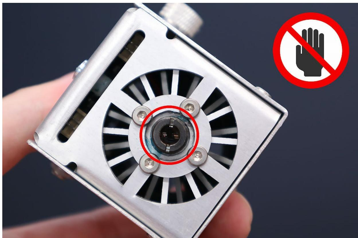
Loosen the screw for laser head height adjustment located on the left side of the laser head. Loosen it until the distance between the laser head and the screw is approximately 2mm.
