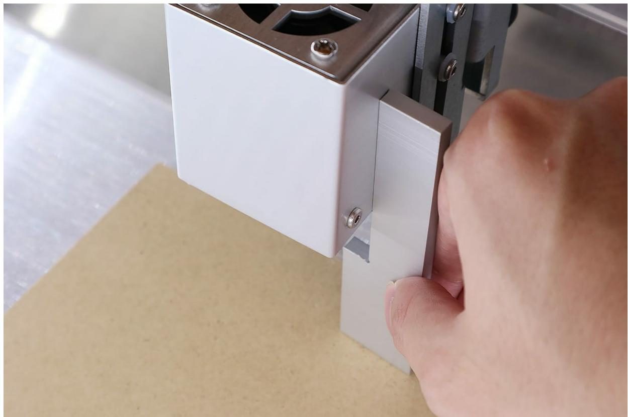
Loosen the screw for height adjustment on the laser head, and slide the laser vertically until the bottom part of the laser head touches the height adjustment jig.
