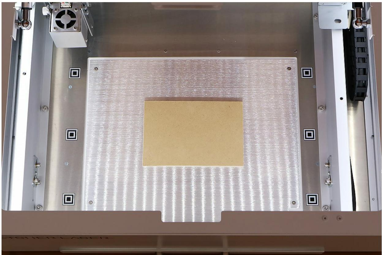
Click the “position check” button, and the graphic area of the software will show the image of the laser head. By dragging the image to a spot, you can move the laser head. Use this function to move the laser head so it is above the material.
