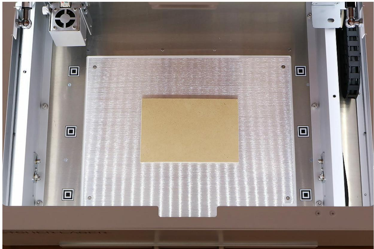
The laser head will move to a certain position when you drag the image of the laser head in the screen to the position you would like to set and tap on “Move”. Use this function to move the laser head so it is above the material. When you finish moving the position of the laser head, tap on “Close”.
