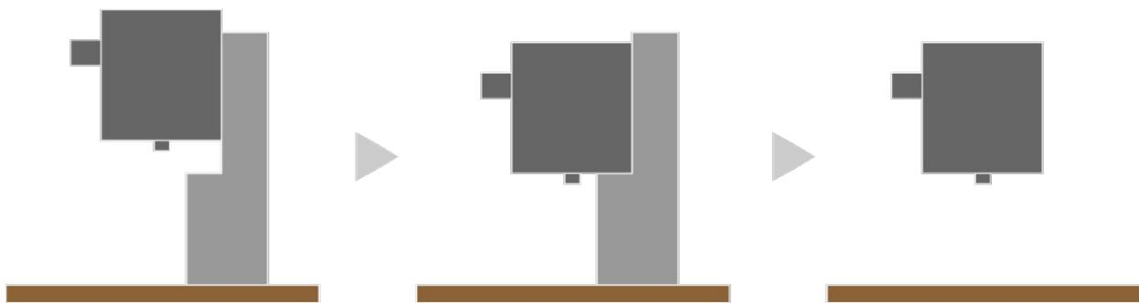
When the height is adjusted, tighten the screw to set the position of the laser head. After that, click the “position check” button again to cancel the position check mode, and click the “Origin” button again to move the laser head to the original position.
