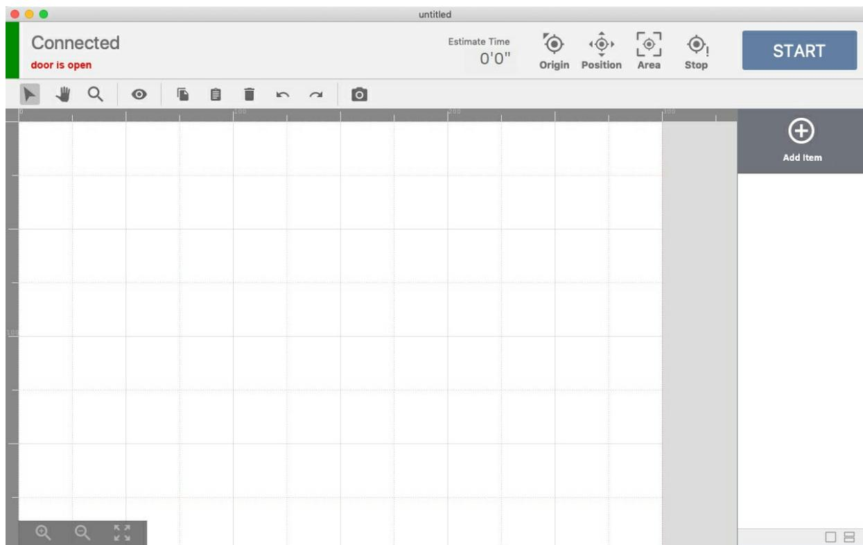
Click the “Origin” on the top of the screen, and the laser head will move to the origin (top left in the work area, default position before it starts processing.)
