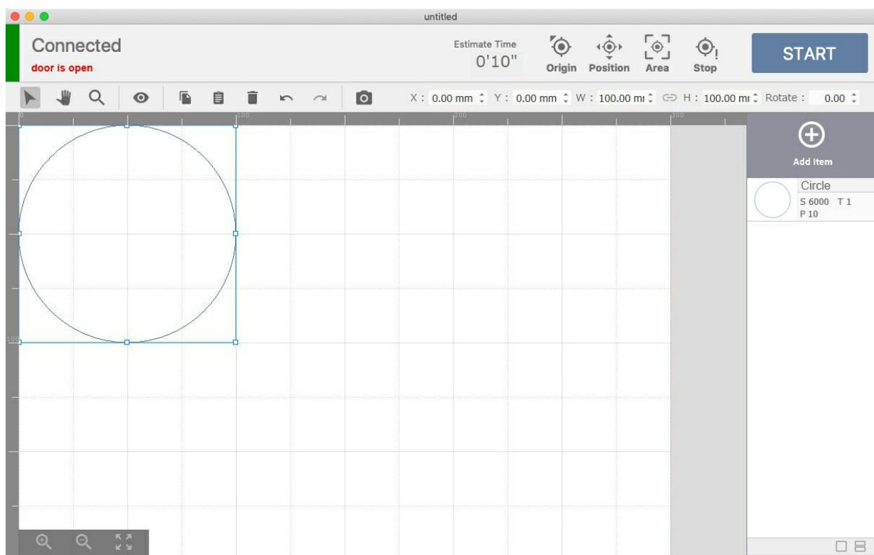
Click the camera icon, the dialog to input the thickness of the material will appear. After you input the number and click the “OK” button, the graphics area will display the material. If the lid is closed and/or the laser head is not positioned on the origin before this step, the material will not appear on the screen properly. The stickers for positioning should not be on the screen. If the stickers are there, redo the step to capture the material by the camera.
