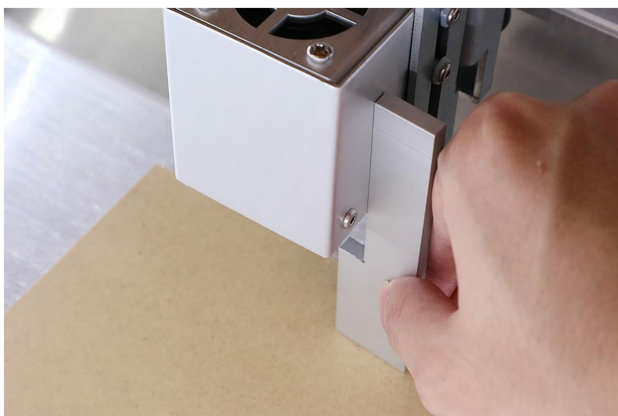
Loosen the screw for height adjustment on the laser head, and slide the laser vertically until
