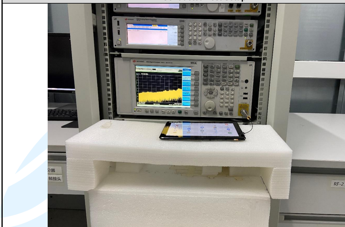
RF Conducted Test Setup
