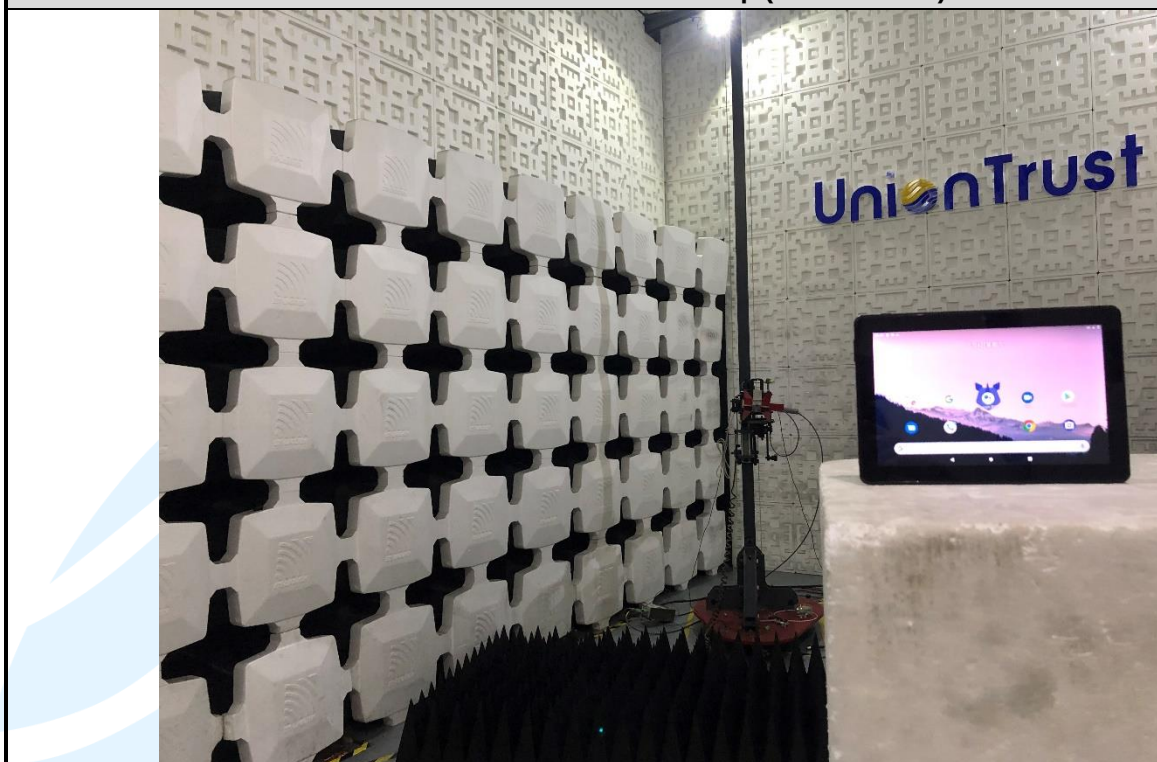
Radiated emission Test Setup (Above 1 GHz)
