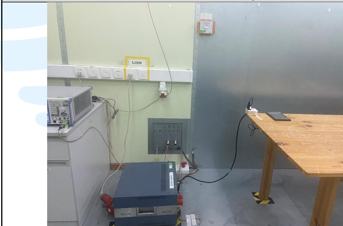
Conducted Emission Test Setup
