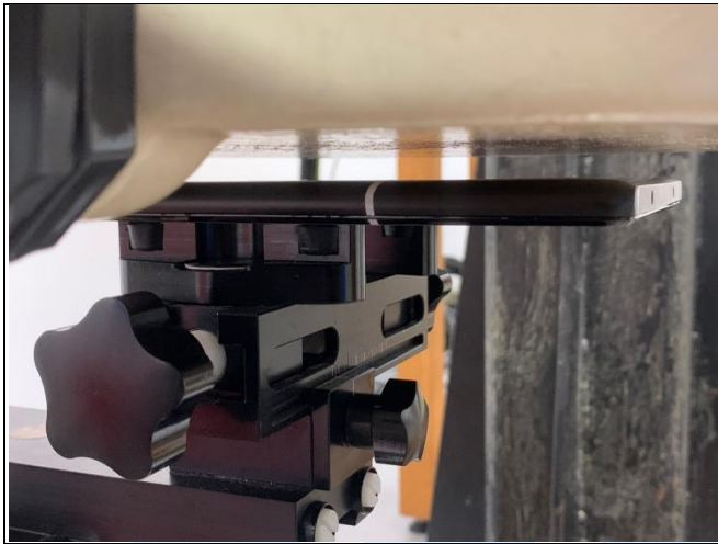
Rear Face of EUT with 10mm Gap
