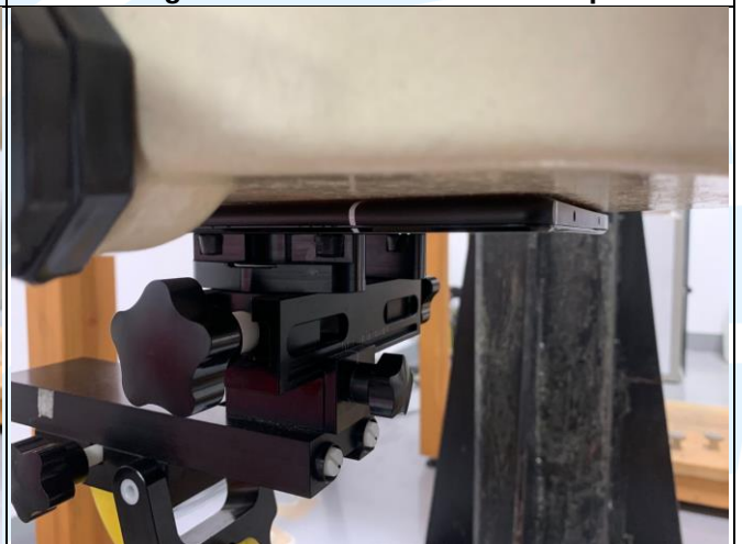
Rear Face of EUT with 0 cm Gap
