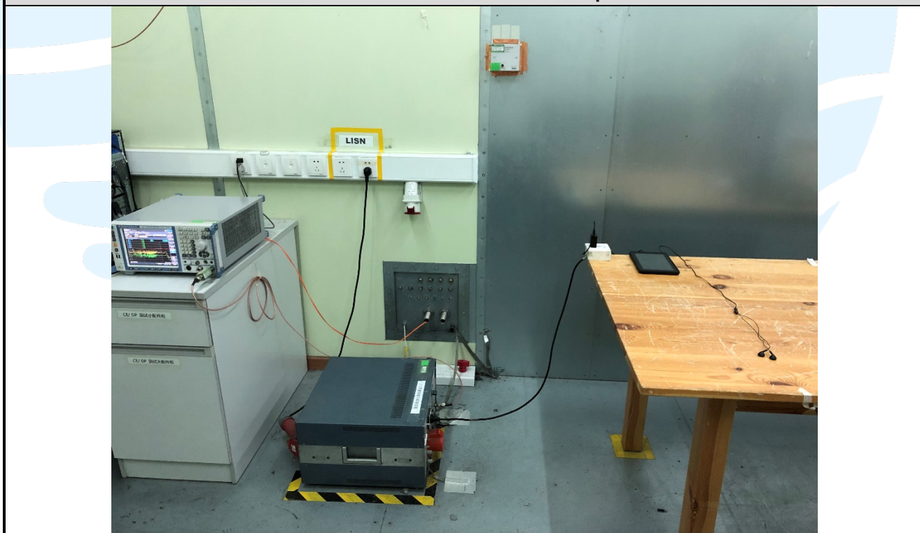
Conducted Emission Test Setup
